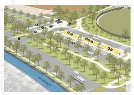
feature a 10-bus bay transit island with pedestrian and bicycle linkages to the central campus, a new signalized intersection on South Campus Drive and amenities such as shade structure with plaza seating, real-time transit information, secured bike parking, water fountains, security cameras, and a bus operator restroom.
