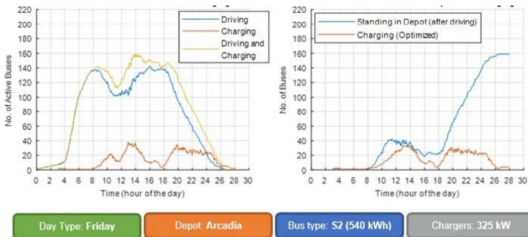
Figure 4-14 shows the number of chargers that are required for bus D3 to operate from Arcadia Yard when using non-optimized charging on the left and optimized charging on the right. Through optimization, the evening peak of the charging curve is flattened. By optimizing the charging, 7 chargers are sufficient instead of 15 chargers that would be required when using non-optimized charging.
