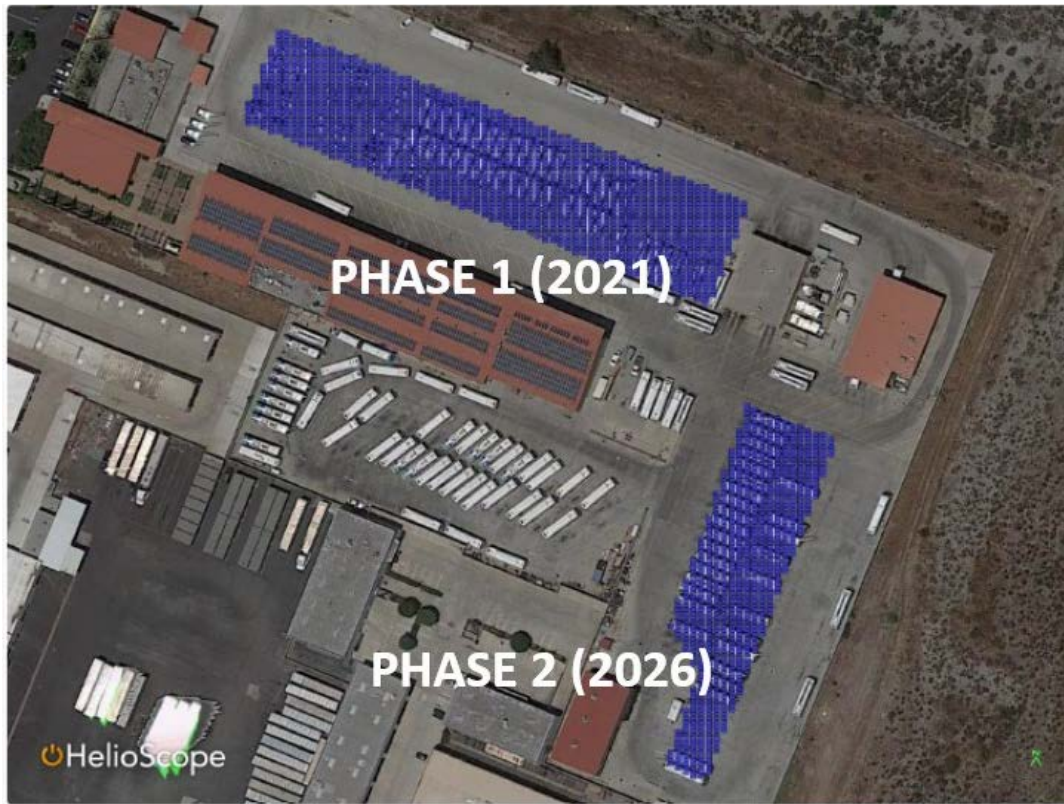
Figure 12-2: Arcadia Depot Solar Layout
