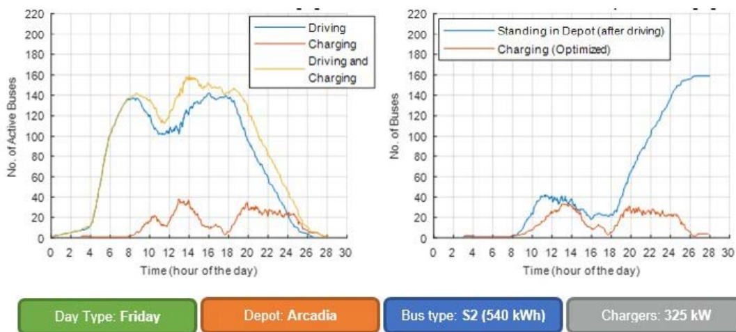
Figure 4-13: Non Optimized Charging Vs Optimized Charging for Bus S2 at Arcadia Yard
